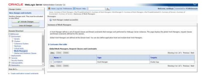
2) Create new Max Thread Constraint and in the Count field give the desired thread count
